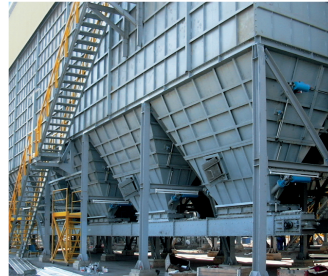
Hoppers with steep inclination avoid dust deposits
