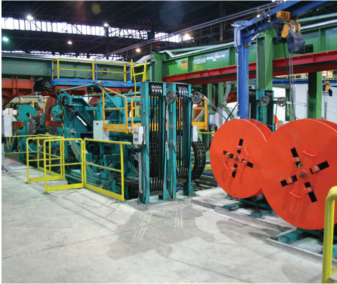
Horizontal compactor with strapping heads
