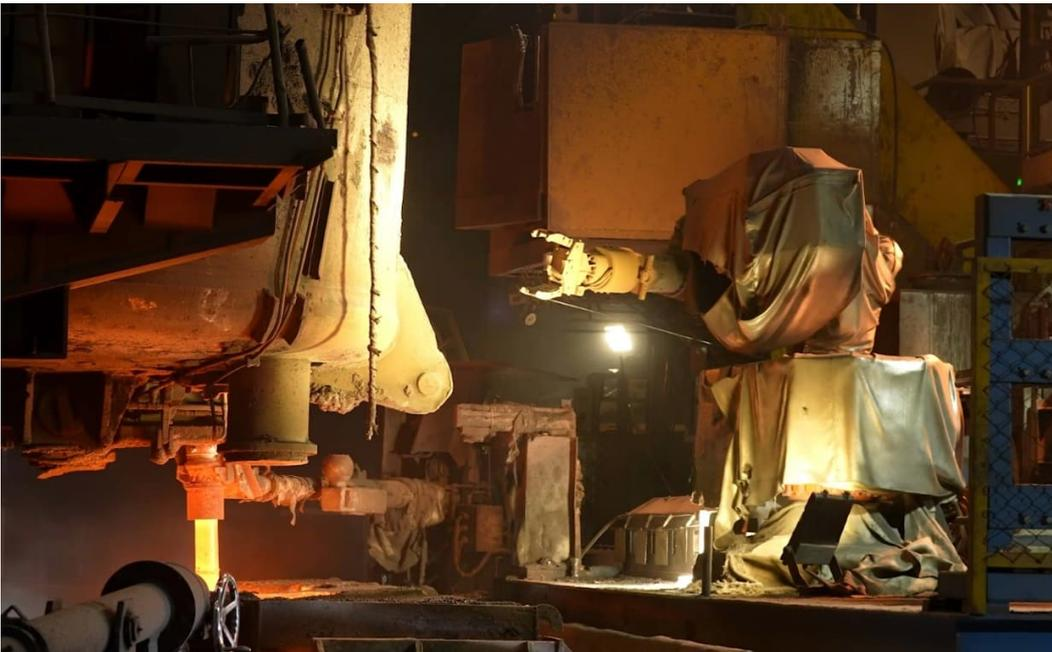
The new tailormade LiquiRob robotics system from Primetals Technologies, in operation at Siam Yamato Steel's plant in Map Ta Phut.
