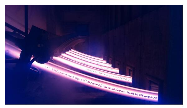
At the minimill of Abinsk Eletric Steel Works in the South Russian region of Krasnodar, Primetals Technologies has modernized the electric arc furnace, the ladle furnace and the 6-strand continuous billet caster. The image shows a 6-strand continuous billet caster from Primetals Technologies.
