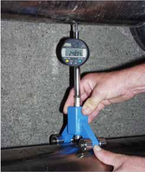
Roll gap measurement with GapChecker
