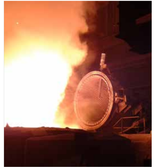
Lomas gas sampling on EAF furnace
