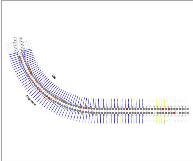
Complete measurement of caster in overview plot showing gap, alignment, roll rotation and spray water distribution.
