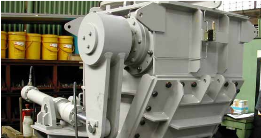
1 | Flap type E&R valve Ø 300 mm
