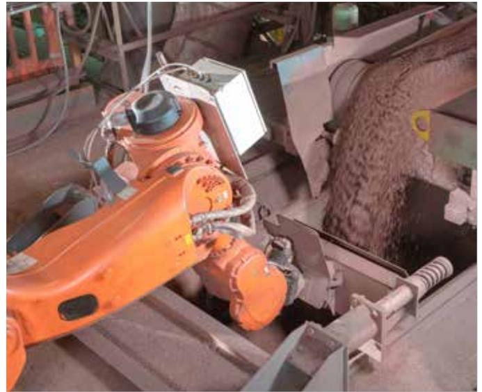
Sinter raw mix sampling during conveyor discharge
