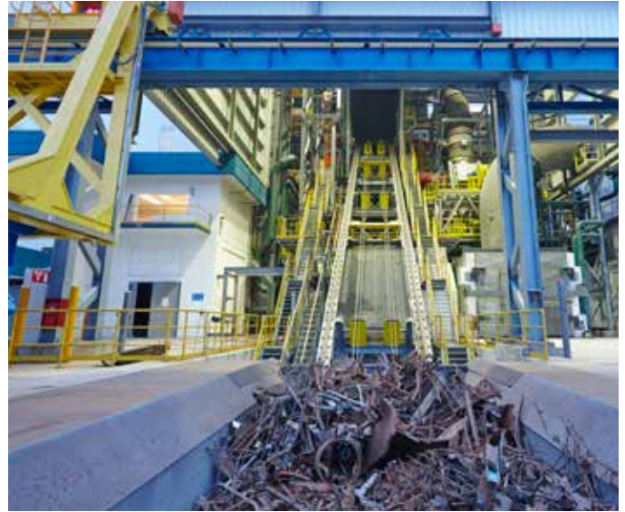
Automated scrap charging system via elevator
