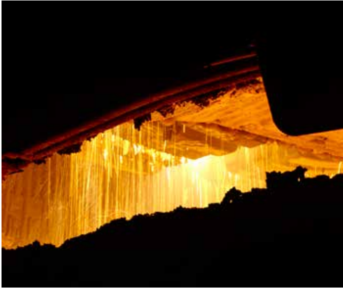
Preheated steel on the finger system
