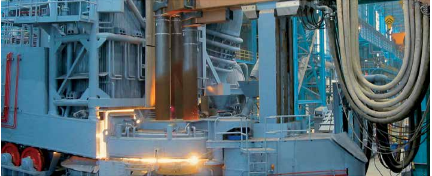
80-t fingershaft furnace in Zhangjiagang, China
