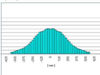
Cumulative water distribution in casting direction
