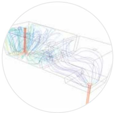
CFD Simulation of tundish flow
