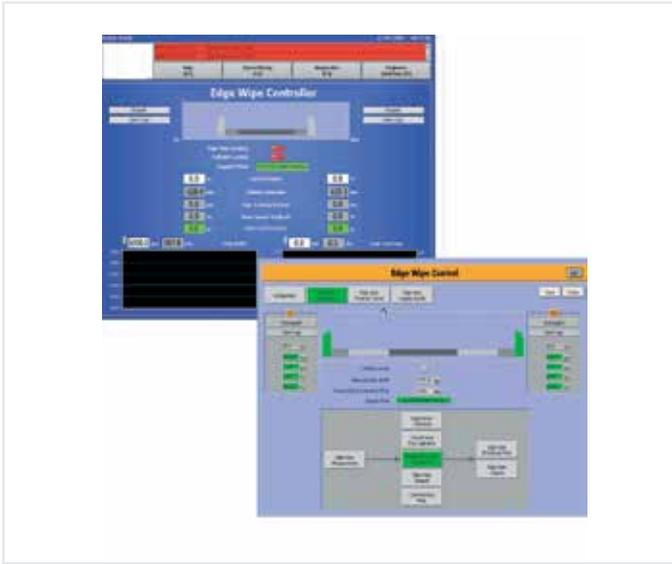
Real time control functionality with integrated HMI and interface screens.
