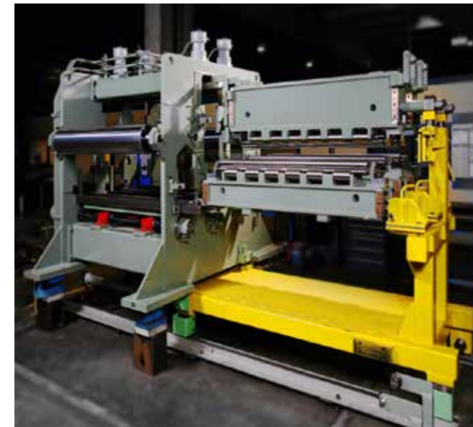
TL 25, Electrolytic galvanizing line
