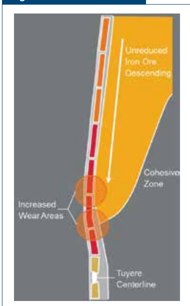
Illustrative example of a potential stave wear cause.
