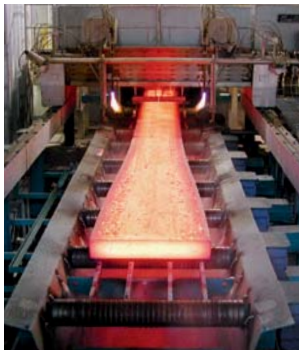
Slab width adjustment with DynaWidth on CC6 at voestalpine Stahl, Austria
