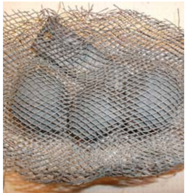
Example of a basket test on briquetted residuals from the direct-reduction process. The tests were performed in the direct-reduction shaft of the DR plant at ArcelorMittal Hamburg, Germany (briquette size: ca. 5 cm 3 )
