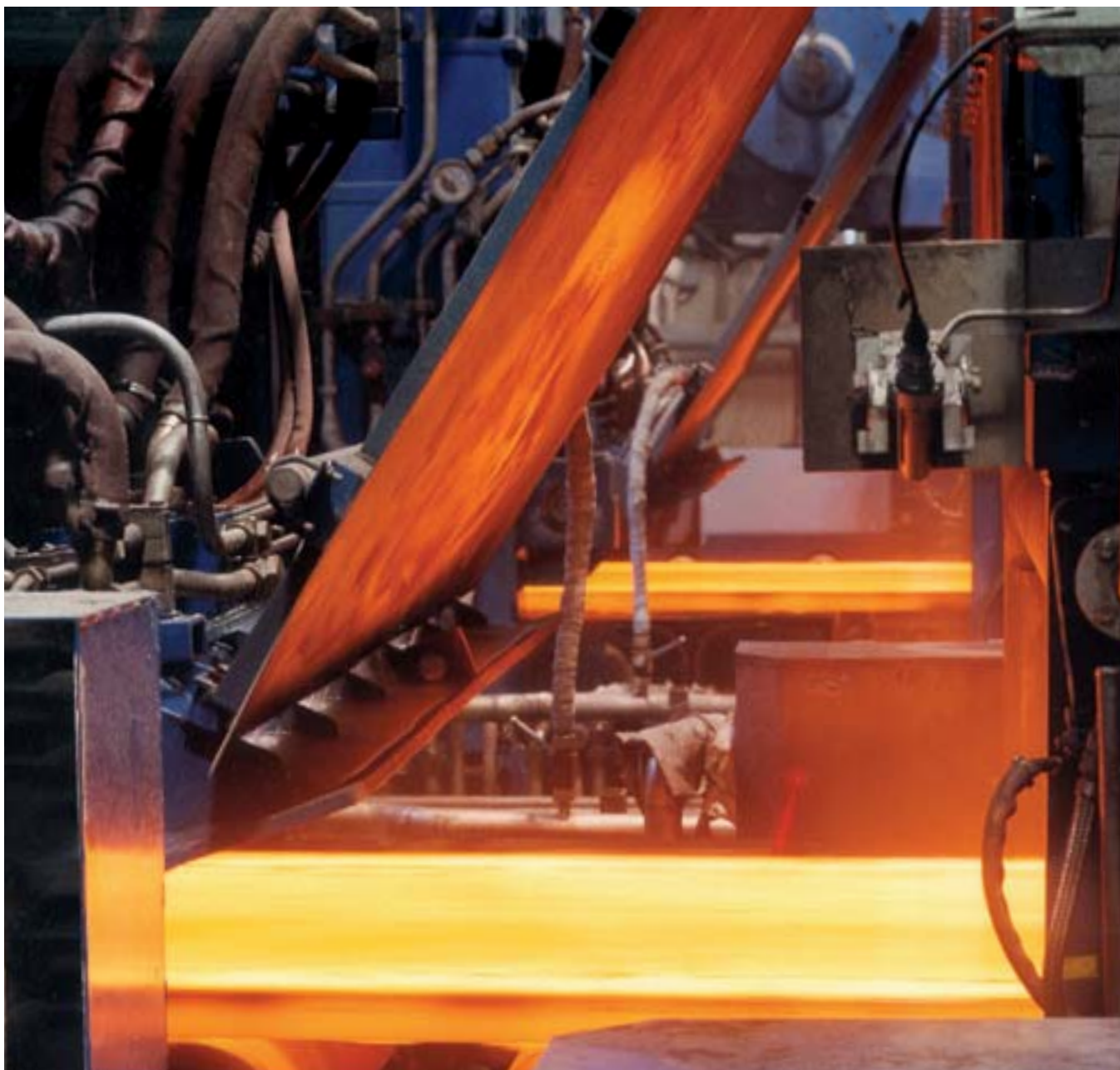
2-strand CSP caster at Bruckhausen, Germany (Copyright by ThyssenKrupp AG 2012)
