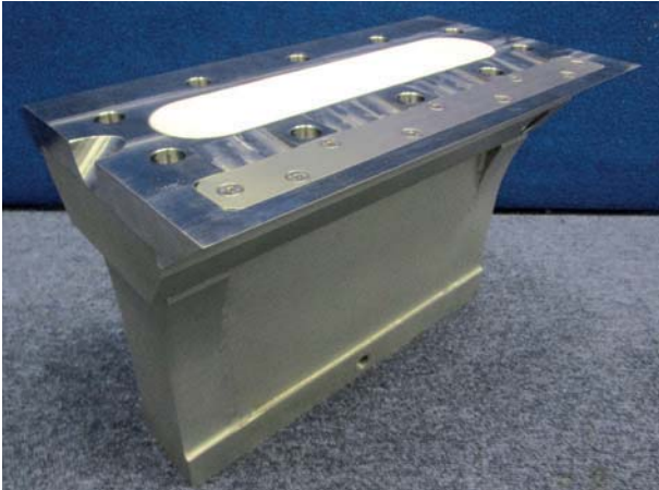
View of an electromagnetic spectroscopy (EMSpec) sensor in the workshop (unit length: approximately 300 mm)
