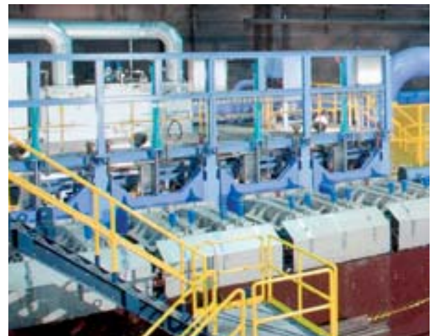
With the Power Cooling solution a wide range of advanced steel grades can be produced in the cooling section of a hot-strip mill
