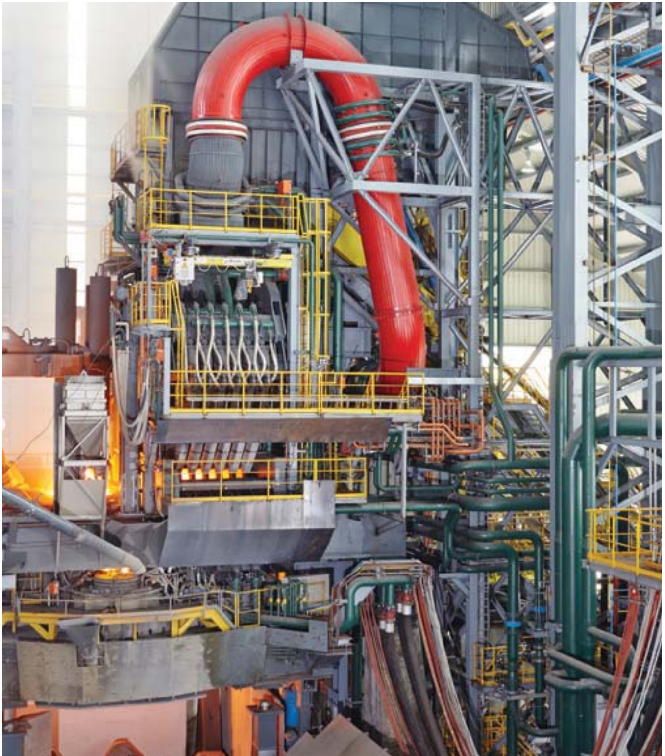
100-ton EAF Quantum Furnace, Tyasa, Mexico
