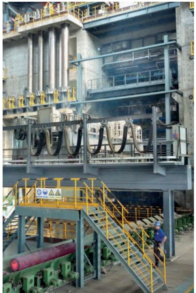
The 2-strand vertical round-bloom caster at Zhongyuan Special Steel Co., Jiyuan, China
