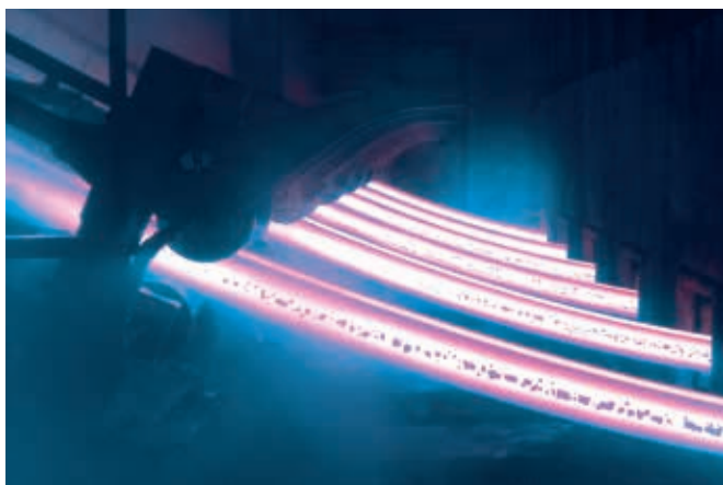
6-strand billet caster in operation at the Abinsk Electrometallurgical Plant
