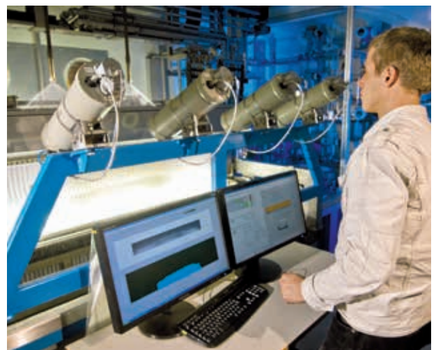
Investigation of the spray performance of different nozzle designs
