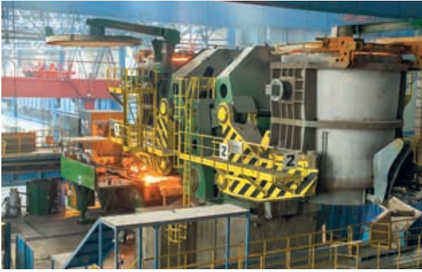
Ladle turret of the Arvedi ESP slab caster at Rizhao Steel, China
