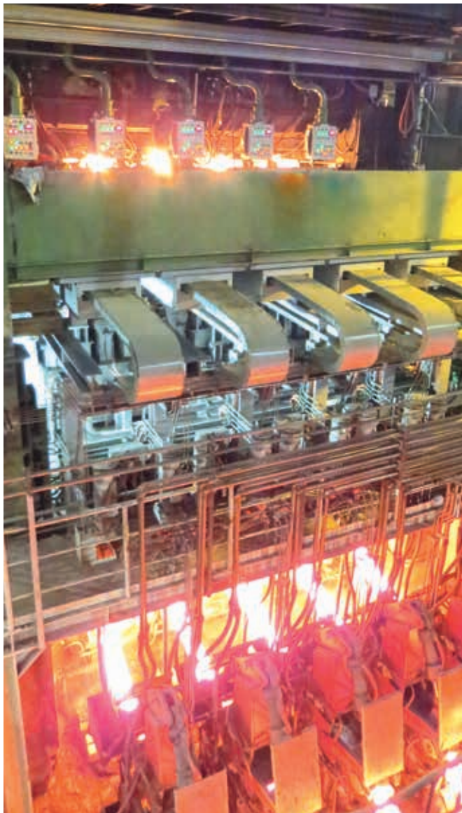
The modernized 5-strand billet caster in operation at ESF Elbe-Stahlwerke Feralpi, Riesa, Germany
