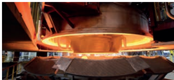
Joint investigation of new vacuum-degassing techniques for the production of high-quality steel grades together with voestalpine Giesserei Linz at the producer's VOD plant in Austria
