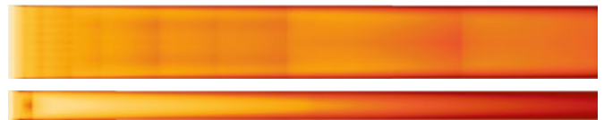
Calculated temperature profile of strand surface (top and side views)
