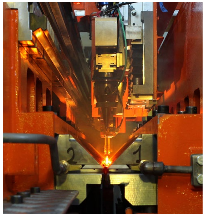
Laser welders supplied by Primetals Technologies France are tested and fine-tuned at the Montbrison Mechatronics Lab prior to installation to ensure optimal operation at the customer's site.
