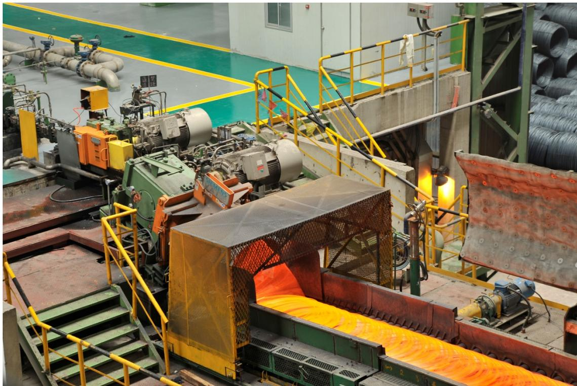
A pinch roll and laying head at Zenith Steel. Primetals Technologies revamps two wire-rod mills for Zenith Steel in Changzhou, China.
