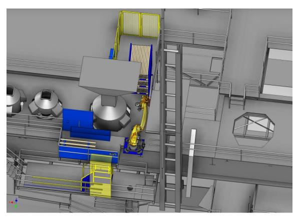
In future, robot systems from Primetals Technologies will manipulate the probes in the three LD (BOF) converters in the voestalpine Stahl Europe steel works in Linz, Austria.
