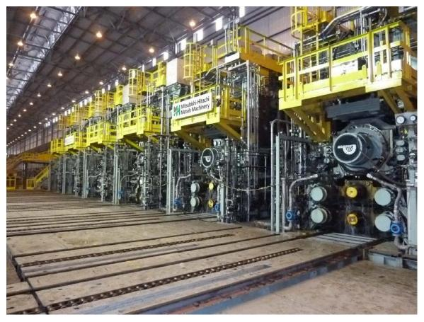
Finishing train of a hot strip mill from Primetals Technologies. The stands are equipped with pair cross technology for optimum control of the profile.
