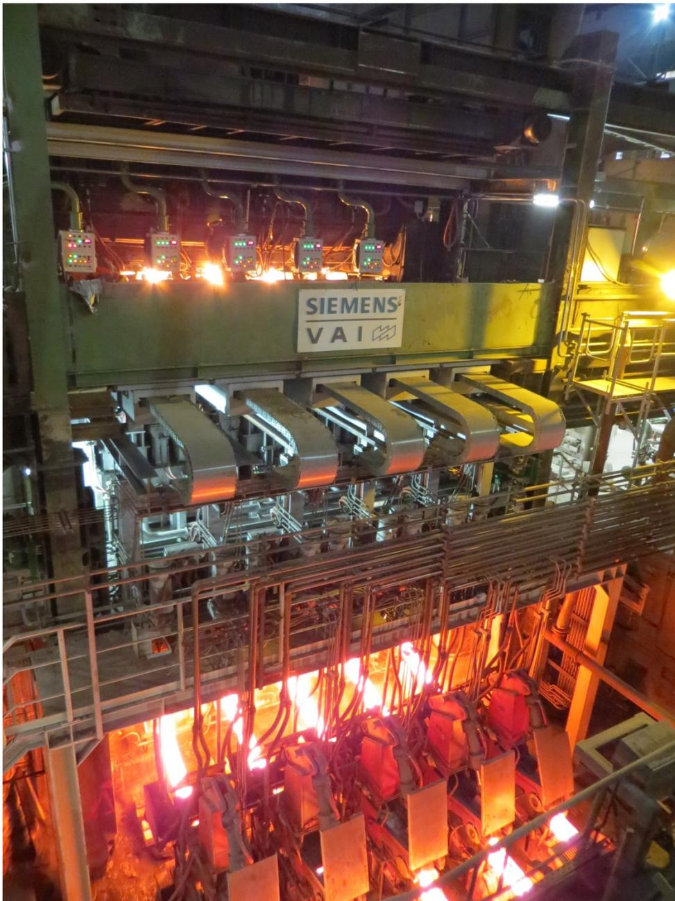
Five-strand continuous billet caster from Primetals Technologies in the Elbe-Stahlwerke Feralpi GmbH (ESF) plant in Riesa, Germany.
