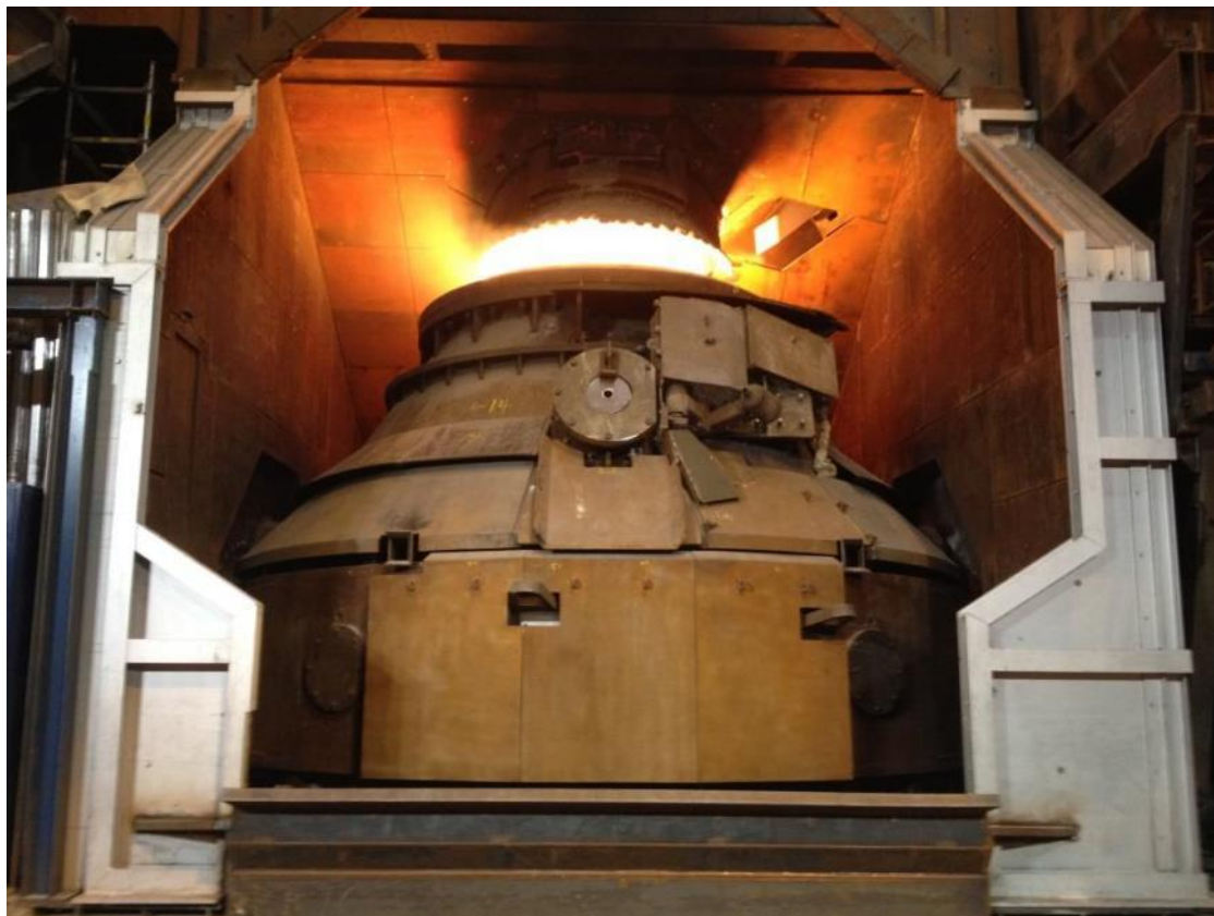
LD (BOF) converter supplied by Primetals Technologies at the Finnish Raahе works of SSAB Europe Oy
