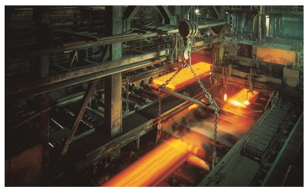
Two-strand continuous slab caster modernized by Primetals Technologies at the German steel producer ArcelorMittal Bremen GmbH (Copyright: ArcelorMittal Bremen GmbH)
