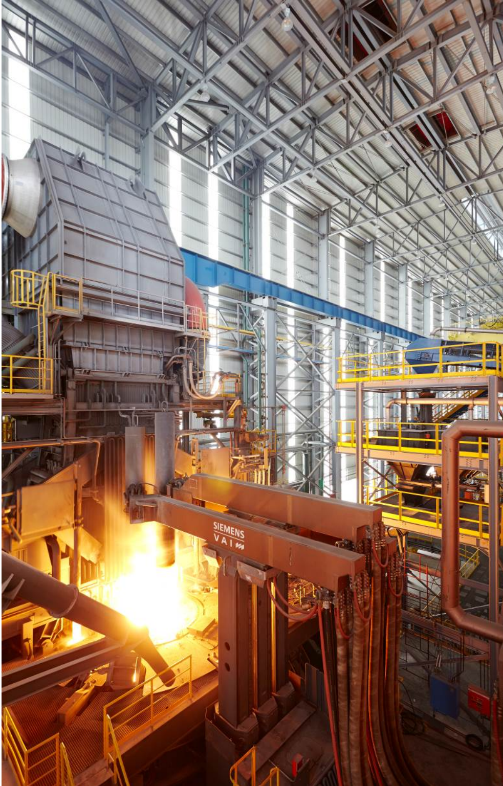
Quantum EAF from Primetals Technologies at Tyasa's minimill meltshop in Ixtaczoquitlan, Mexico
