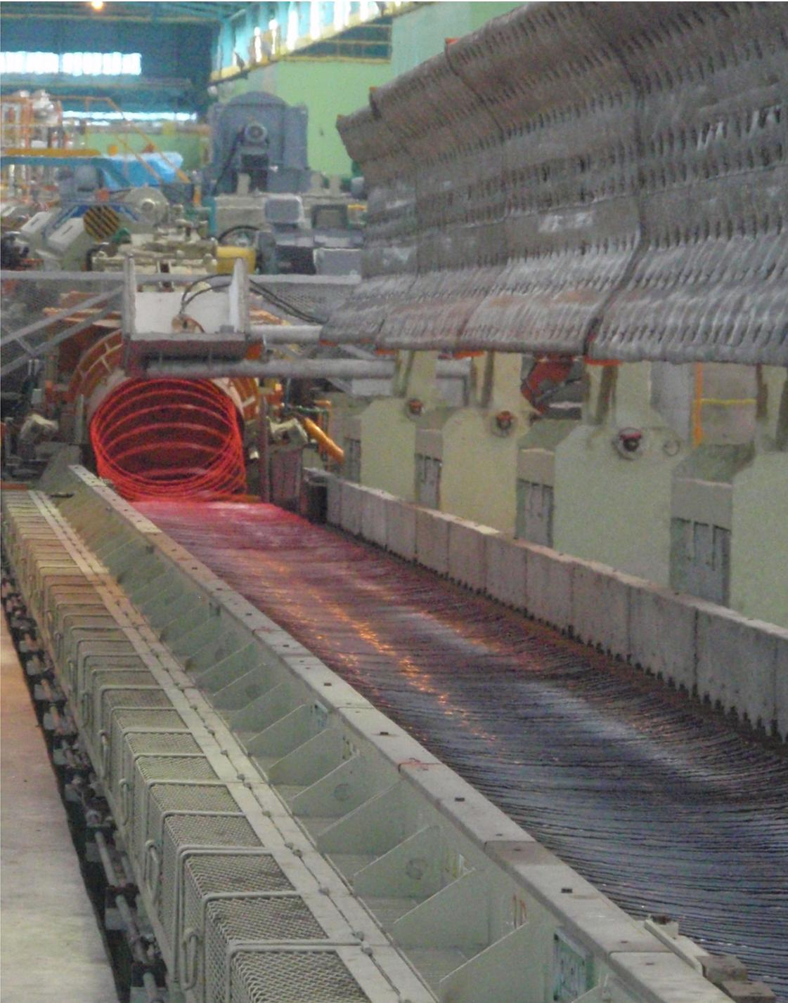
Morgan Stelmor Cooling Conveyor operating with Optimesh system from Primetals Technologies beneath nozzle deck. Optimesh ensures cooling uniformity for high carbon products in fast cooling mode. The system will be installed in a wire-rod outlet of Zenith Steel in China.
