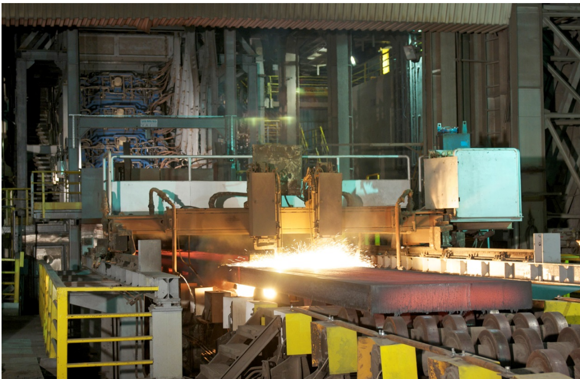
Continuous caster of at Acroni, d.o.o. in Jesenice, Slovenia. The caster was modernized by Primetals Technologies and now also produces X120 Mn12 grades.
