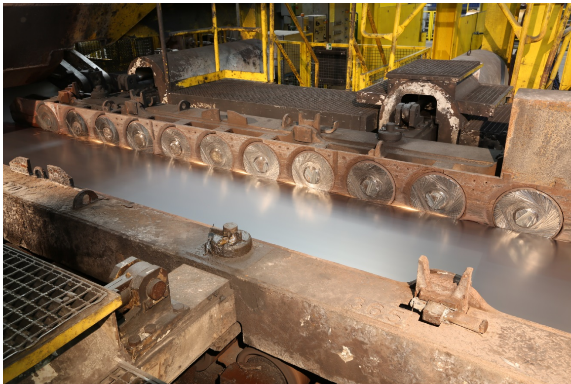
Side guides with Eco Slide Discs from Primetals Technologies at the entry side of the down coiler in the hot strip mill of voestalpine Stahl in Linz, Austria.
