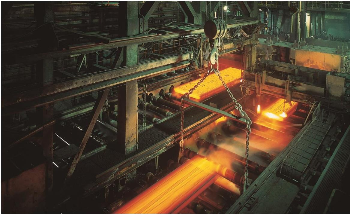
Two-strand continuous slab caster modernized by Primetals Technologies at the German steel producer ArcelorMittal Bremen GmbH (Copyright: ArcelorMittal Bremen GmbH)
