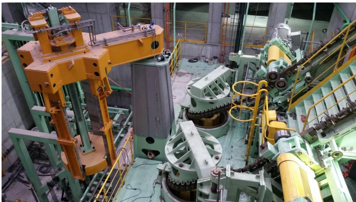
Two pouring reels and transfer mast for bar in coil products from Primetals Technologies
