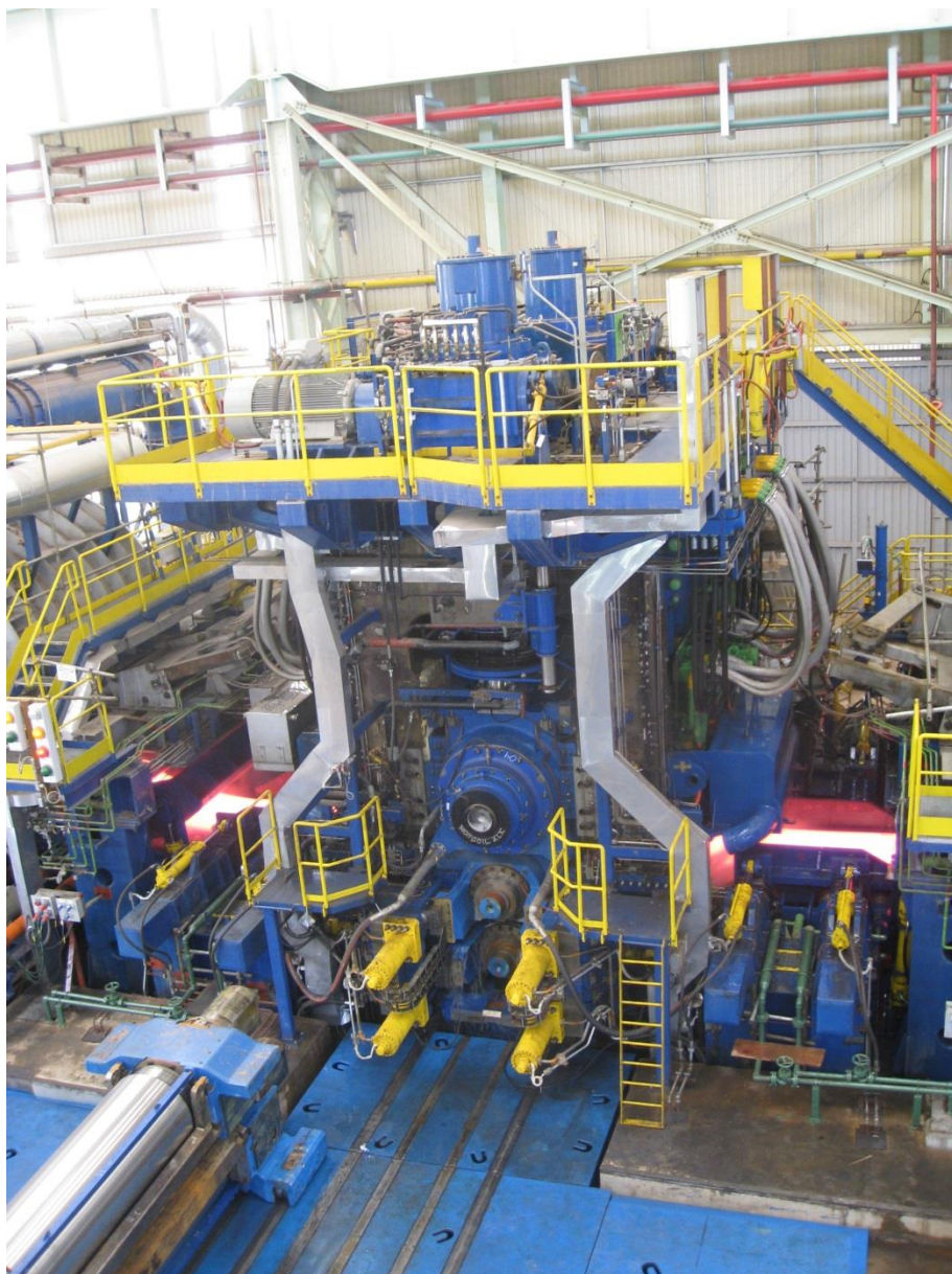
Steckel mill supplied by Primetals Technologies for the Ouro Branco production site of Brazilian steel producer Gerdau Ouro Branco in the state of Minas Gerais
