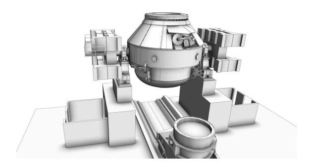
Computer-animated depiction of an LD (BOF) converter from Primetals Technologies to be installed for ArcelorMittal Poland in the Dabrowa Górnicza steel works
