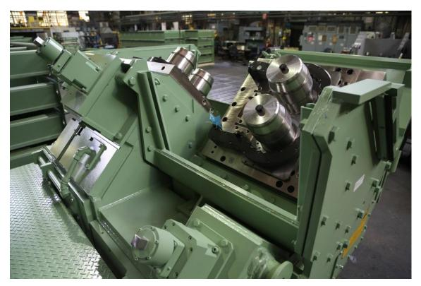
Highest capacity 250 mm ultra heavy-duty (UHD) roll unit for high speed wire rod mills from Primetals Technologies prior to shipment.
