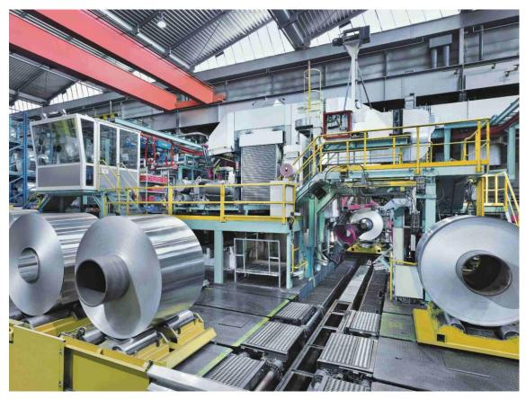
Aluminum strip production at AMAG rolling GmbH in Ranshofen, Austria. Primetals Technologies is modernizing the drive technology of the four-high cold rolling stand (photo: AMAG rolling GmbH)
