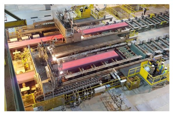
Two-strand continuous slab caster from Primetals Technologies in the Brazilian steel works of Companhia Siderúrgica do Pecém (CSP). The caster is part of a new plant in the Pecém Industrial and Port Complex in São Gonçalo do Amarante in the state of Ceará.
