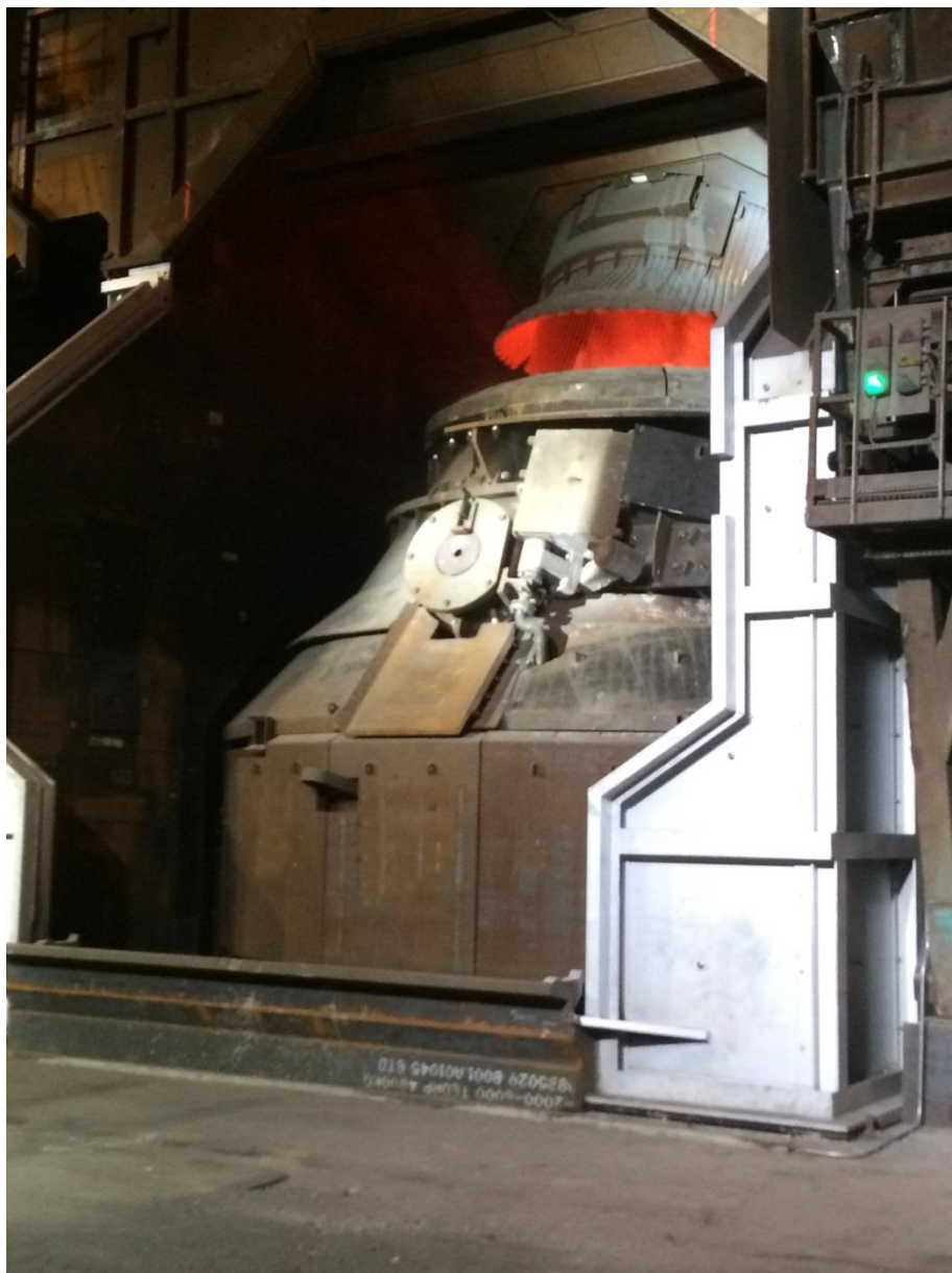
LD (BOF) converter supplied by Primetals Technologies at the Finnish Raahe works of SSAB Europe Oy
