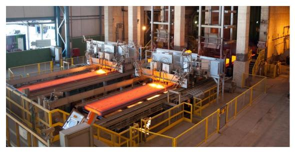
Twin-strand continuous slab caster from Primetals Technologies. Two comparable machines will be supplied to Chinese steel producer Shandong Iron & Steel Group Rizhao Co., Ltd.
