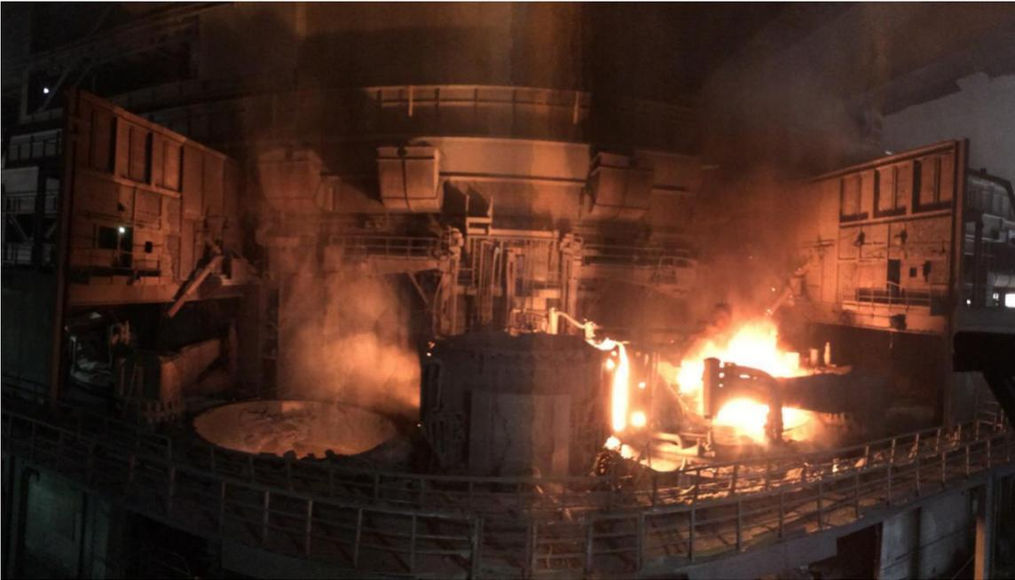
150-metric-ton twin electric arc furnace at Baosteel in Shanghai, China. The furnace will be modernized by Primetals Technologies by the end of 2016.
