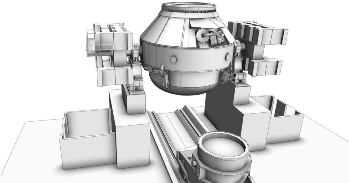
Computer-animated depiction of an LD (BOF) converter from Primetals Technologies to be installed for ArcelorMittal Poland in the Dąbrowa Górnicza steel works
