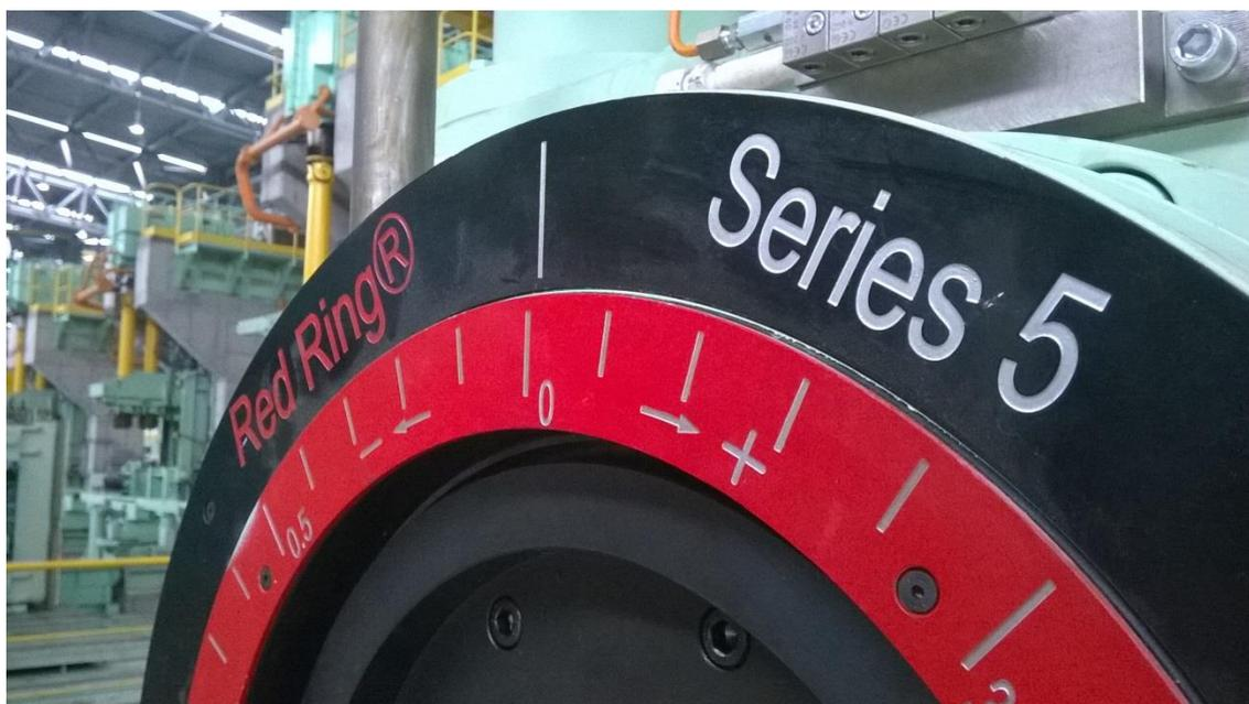
Series 5 Red Ring rolling stand from Primetals Technologies. Two of these stands were installed on the roughing train of the bar mill of Hennigsdorfer Elektrostahlwerke GmbH (H.E.S).
