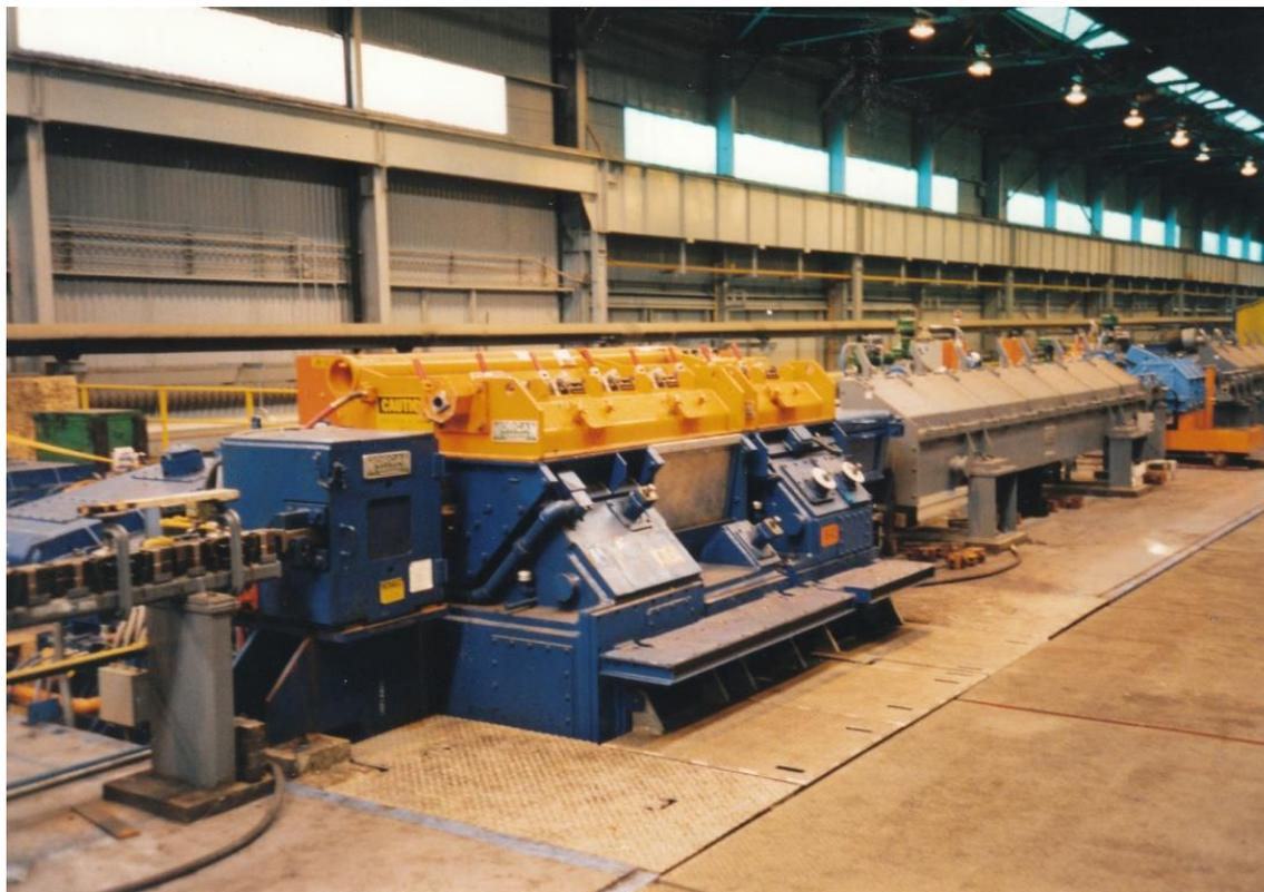
A Morgan Reducing/Sizing Mill from Primetals Technologies in a wire rod mill.
