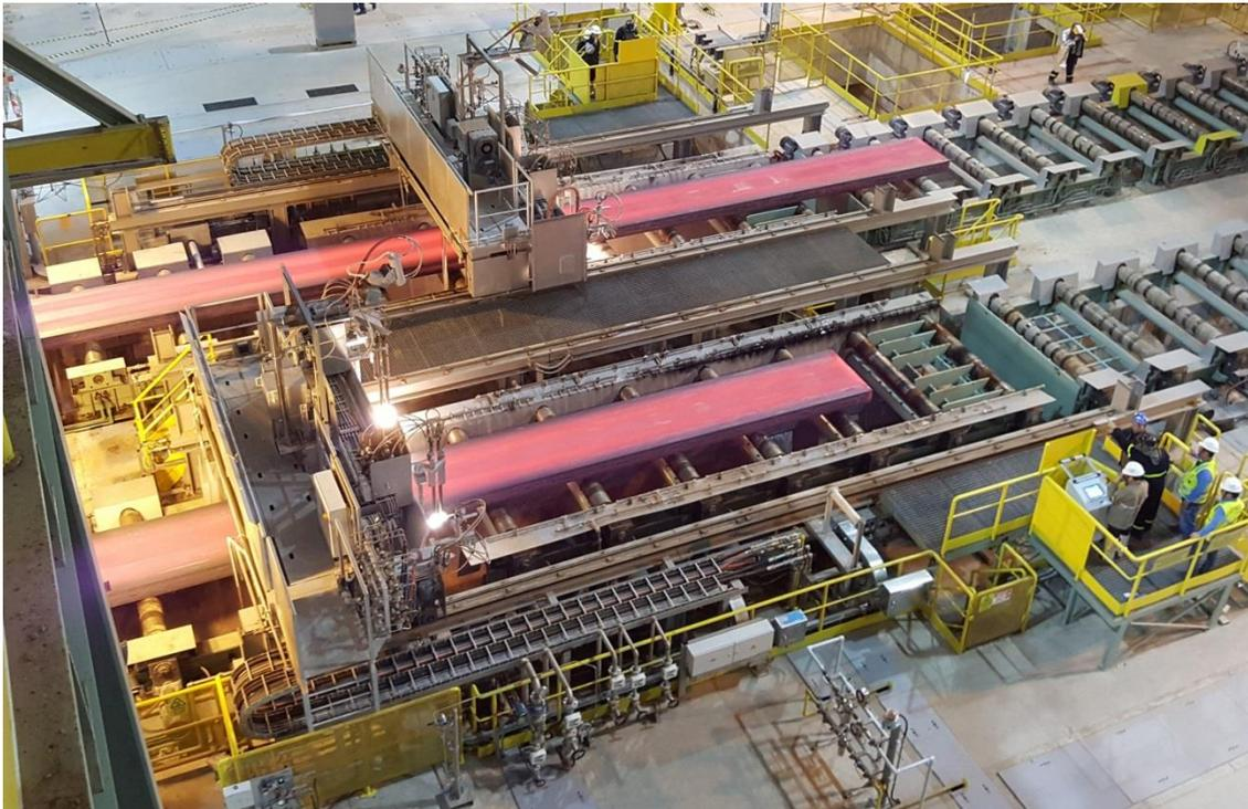
Two-strand continuous slab caster from Primetals Technologies in the Brazilian steel works of Companhia Siderúrgica do Pecém (CSP). The caster is part of a new plant in the Pecém Industrial and Port Complex in São Gonçalo do Amarante in the state of Ceará.
