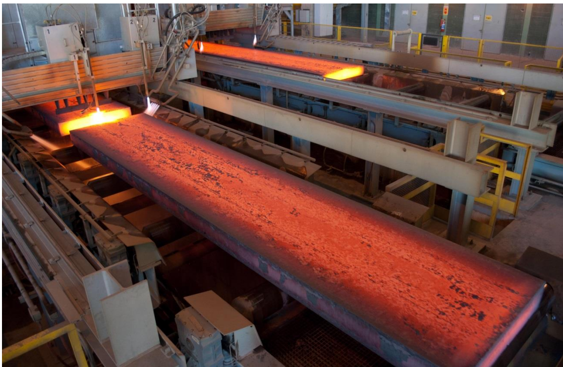
Slabs produced on a continuous casting machine from Primetals Technologies
